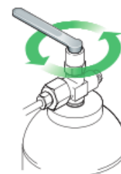
Turn anticlockwise to open key operative valve
